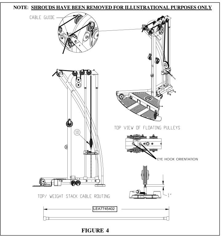
MUST DISASSEMBLE ONE END OF CABLE AND REASSEMBLE AFTER ROUTING (SEE FIG 7 PAGE 14)
